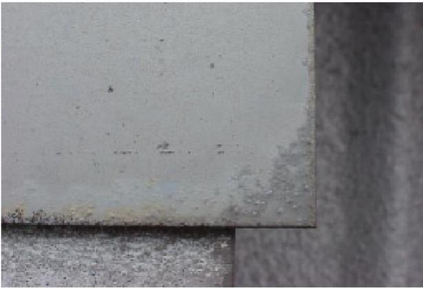
*Under film corrosion on a coil coated section of galvanized steel. Exposed on GI roof for 15 years.*
