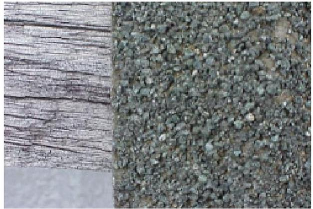
*Edge of Al Zn steel acrylic tile. Exposed on GI roof for 22 years.*
