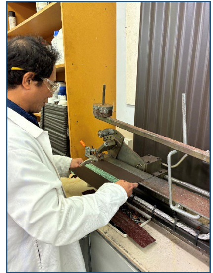
Figure 4: Gerard Chemist Performing a Scrape Test
