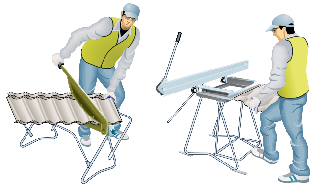
Figure 6.2.7.2 Valley tile being cut then bent
