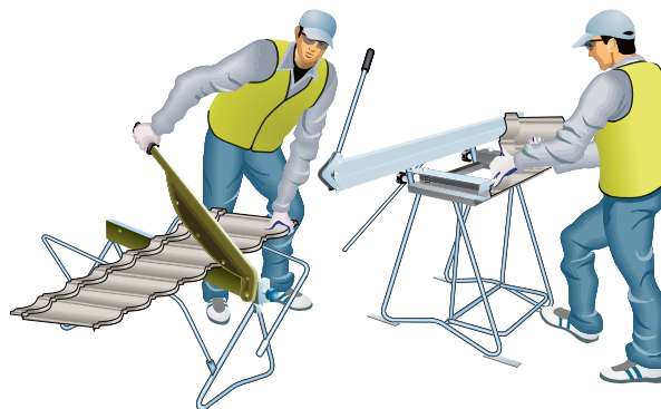
Fig 6.2.5.3 Hip tile being cut then bent
