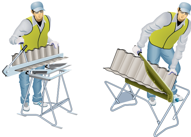
Figure 14.7.6.3 Ridge tile being bent then cut
