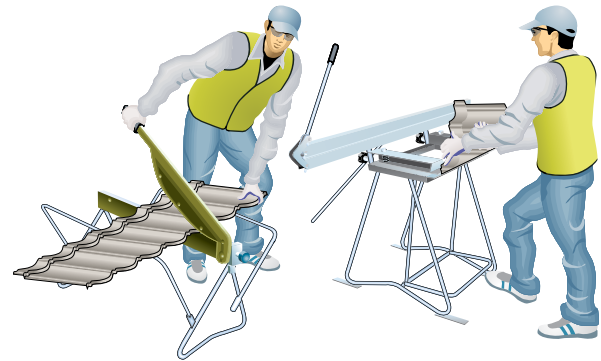
Figure 14.7.5.2 Cutting and bending a hip tile
