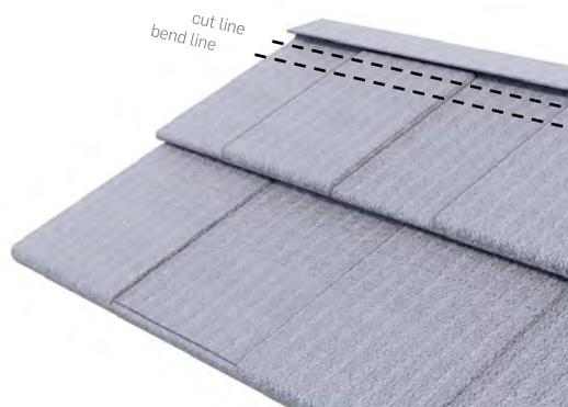
Cut your panel along the cut line. Then bend the head of the panel to create a minimum of 40mm upstand against the wall or support nog.
