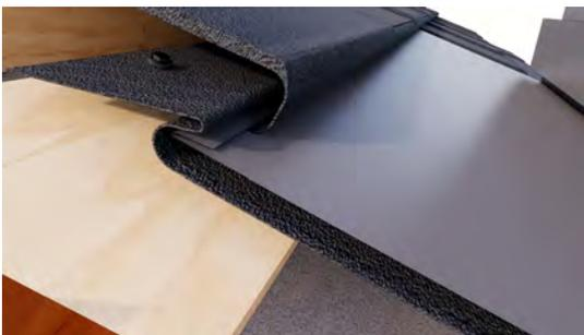
If the distance from the back of the chimney to the batten is less than 150mm, extend your back flashing up to the next batten.
