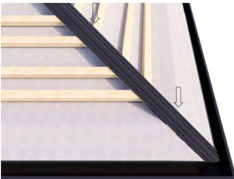
Screws or nails should be fixed to the battens through the farthest edge, avoiding the weather channels.
