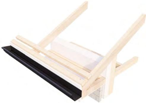
Fix the eaves flashing into the first batten with a minimum 40mm overhang from the fascia into the gutter. Fix with a fastener every 400mm across the eaves flashing.
