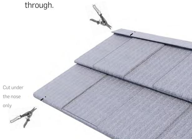
Then bend the side end of the panel to create a 40mm upstand. When installing the next course, add a bead of silicone to the join.
