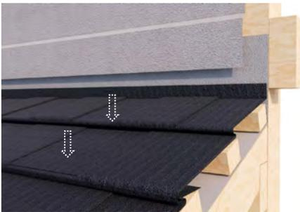
Fix the side flashing to the support nog in the wall. Wall underlay should lay over the top of the side flashing.
