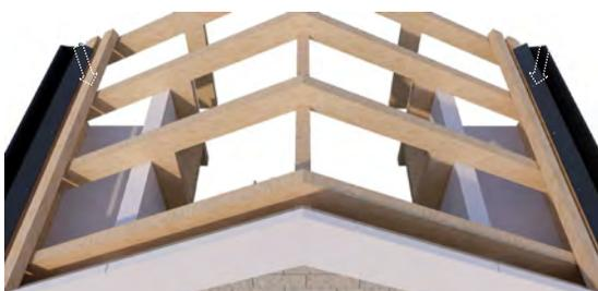
Install underlay across the roof and fasten 40x50mm battens over the underlay. Underlay should be draped over the top of the already-installed batten/s at the eaves.
