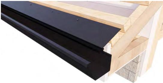
Pinout and fix underlay to the roof, with the overlay on top of the already fixed batten/s and eaves flashing. Underlay should finish 10mm short of the edge of the eaves flashing.
