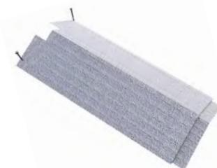
Hook the next trim into the installed trim's head and fasten, making your way up the hip.
