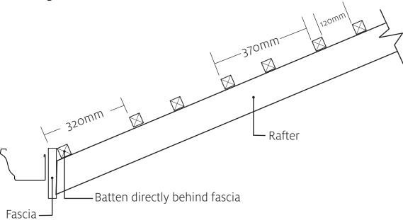
The first batten is spaced 320mm from the front of the fascia to allow a 50mm overhang into the gutter.
