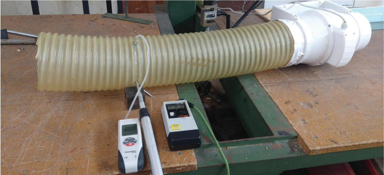
Ducting, fan, manometer and anemometer
