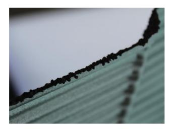
Stone granules at the edge of a tile, this may be removed during installation and handling. This chip may end up being washed down into the gutter.
